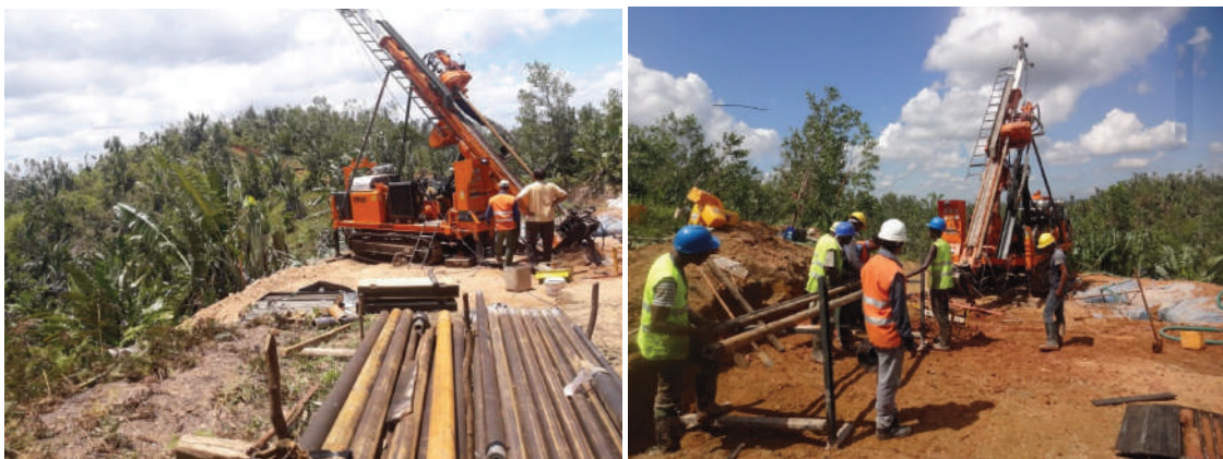
Core drilling in progress at Vatomina
