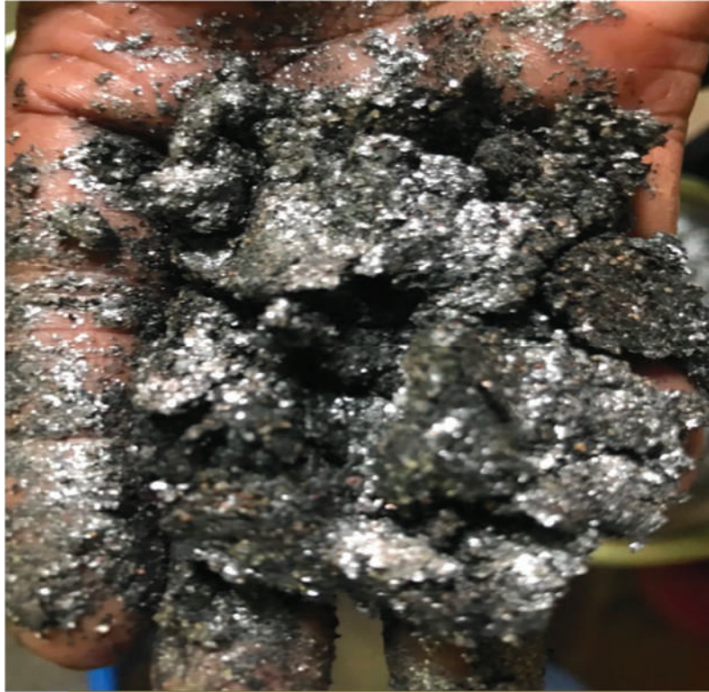
Flake Graphite concentrate produced during metallurgical tests
