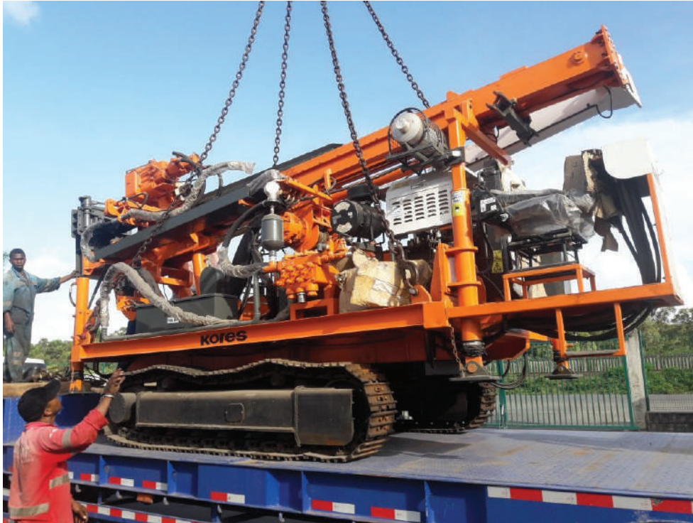
Track mounted diamond core drilling machine at Madagascar on arrival
